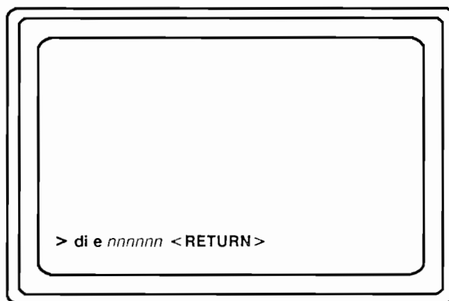
Figure 8-29. Directing the Memory Dump Across the Network
