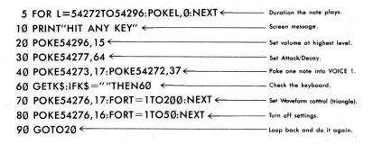
Here, we're using VOICE 1 to create one note at a time . . . with a MEDIUM ATTACK RATE and ZERO DECAY. The key is Line 40. POKEing the ATTACK/DECAY setting with the number 64 activates a MEDIUM attack rate. The result sounds like someone bouncing a ball in an oil drum. Now for the fun part. Hit the RUN/STOP key to stop the program, then type the word LIST and hit RETURN. Now type this line and hit RETURN (the new line 40 automatically replaces the old line 40):
