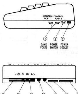
(1) 6 AUDIO/VIDEO SERIAL CASSETTE CONNECTOR PORT INTERFACE CARTRIDGE CHANNEL USER TV
