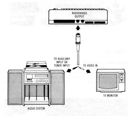
If you purchased peripheral equipment, such as a VIC 1541 disk drive or a VIC 1515 printer, you may wish to connect it at this time. Refer to the user's manuals supplied with any additional equipment for the proper procedure for connecting it to the computer. A completed system might look like this.
