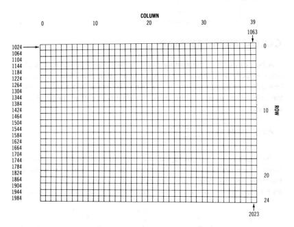
Screen memory in the Commodore 64 normally begins at memory location 1024, and ends at location 2023. Location 1024 is the upper left corner of the screen. Location 1025 is the position of the next character to the right of that, and so on down the row. Location 1063 is thé right-most position of the first row. The next location following the last character on a row is the first character on the next row down.
