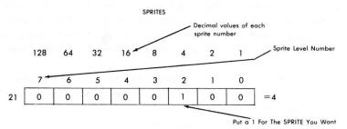
Each sprite level is represented in section 21 of the sprite memory and 4 happens to be sprite level 2. If you were using level 3 you would put a 1 in sprite 3 which has a value of 8. In fact if you used both sprites 2 and 3 you would put a 1 in both 4 and 8. You would then add the numbers together just like you did with the DATA on your graph paper. So, turning on sprites 2 and 3 would be represented as V+21,12.
